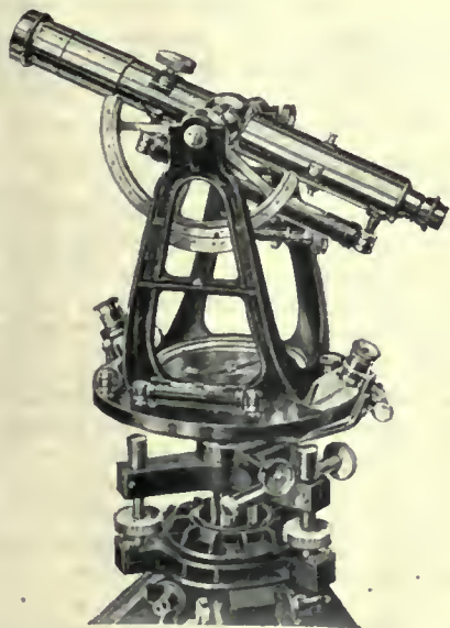
AINSWORTH, TYPE 'A 3W', PRECISION THEODOLITE.
